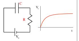
b.) Noting that because the cap is charging, i = +dq/dt, it's differential equation is shown below.
