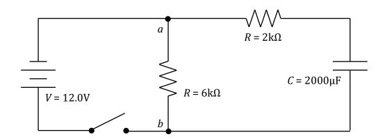
The switch is opened again, and a 6000 $\Omega$  resistor placed across the circuit from point a to point b at a new time t = 0.
