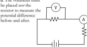
b. The ammeter must be inserted into the circuit so that there is only one path for current to follow. The ammeter may be placed anywhere in the circuit to measure current because it's a series circuit and the current is the same everywhere. But it make s most sense intuitively to place the meter near the resistor.
