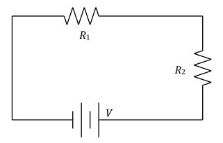
10. Two resistors are placed in series with a battery of potential V as shown above.
