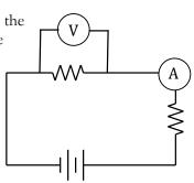
c. The two resistors are in series, so the current *I* is the same throughout the circuit. Using Ohm's Law and the information we have for *R*<sub>1</sub>:
