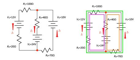
We have three unknown currents— $I_1$ ,  $I_2$ , and  $I_3$ —so we'll need three equations to be able to solve simultaneously.
