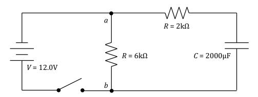
The switch is opened again, and a  $6000\Omega$  resistor placed across the circuit from point a to point b at a new time t = 0.
