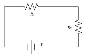
2. Two resistors are placed in series with a battery of potential V as shown above.
