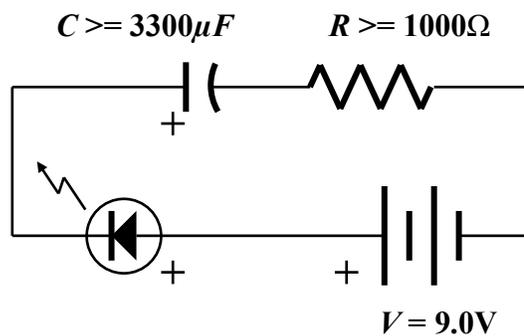
1. Build the circuit shown here. Note that capacitor and the LED both have one longer lead that indicate their *anodes*, which need to be connected to the positive (+) end of the circuit. If using a breadboard, you may find it convenient to refer to the photo at the end of this handout.
