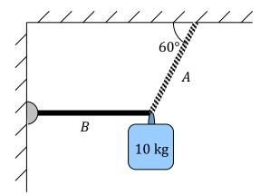
A mass of 10 kg is suspended from a cable A and a light, rigid, horizontal bar B that is free to rotate, as shown. What is the approximate tension, in Newtons, in cable A?
