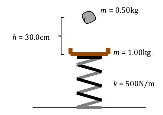
Now the platform is placed again at its equilibrium position. A 500 gram blob of clay is released from a height of 30.0 centimeters above the platform so that it falls and contacts the platform in a perfectly inelastic collision.
