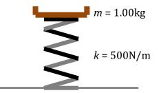
A spring of negligible mass and spring constant 500 N/m is oriented vertically as shown. A flat 1.00 kg platform is then attached to the top of the spring.
