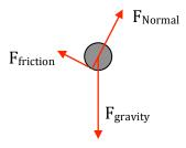
Note that the Normal force should originate from the point where the cylinder touches the surface, as should the force of Friction acting parallel to the plane. The force of gravity should originate at the center of mass of the cylinder.
