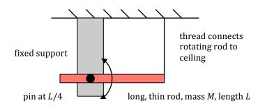
A long, thin, rod of mass M = 0.500kg and length L = 1.00 m is free to pivot about a fixed pin located at L/4. The rod is held in a horizontal position as shown above by a thread attached to the far right end.
