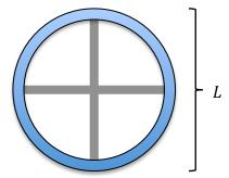
A pair of long, thin, rods, each of length L and mass M, are connected to a hoop of mass M and radius L/2 to form a 4-spoked wheel as shown above. Express all answers in terms of the given variables and fundamental constants.
