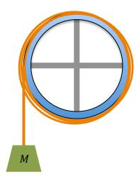
The wheel is now mounted to a frictionless fixed axle and suspended from a vertical support. Several turns of light cord are wrapped around the wheel, and a mass M is attached to the end of the cord and allowed to hang. The mass is released from rest.
