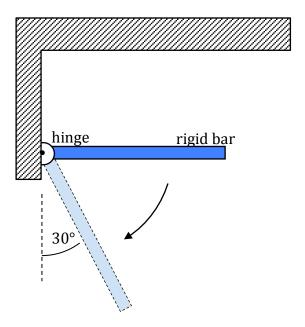
A rigid bar with a mass M and length L is free to rotate about a frictionless hinge at a wall. The bar has a moment of inertia  $I = 1/3 ML^2$  about the hinge, and is released from rest when it is in a horizontal position as shown. What is the instantaneous angular acceleration when the bar has swung down so that it makes an angle of 30° to the vertical?
