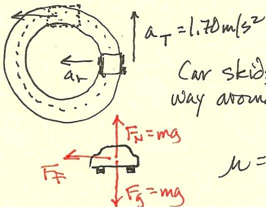
Car skids off after  $\frac{1}{4}$  of the way around the track. Calculate  $\mu_s$ .
