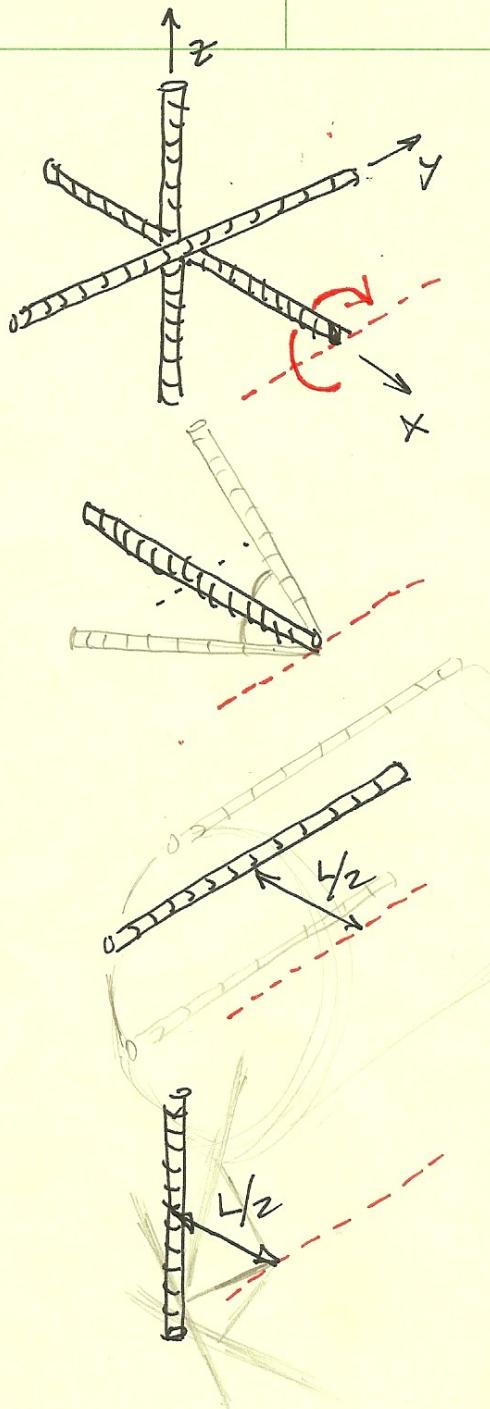
Find  $I_{\text{total}}$  for the 3-rod assembly shown, & rotated about a line parallel to the y-axis at one end of the rods.
