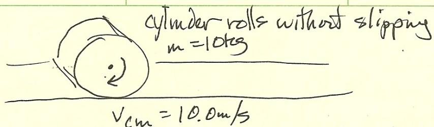
a)  $K_{\text{translational}} = \frac{1}{2} M V_{cm}^2 = \frac{1}{2} (10 \text{ kg}) (10 \text{ m/s})^2 = \boxed{500 \text{ J}}$
