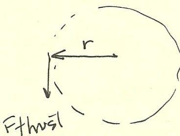
$$\text{a) } \tau = r \times F = (30 \text{ m})(0.800 \text{ N}) = \boxed{24.0 \text{ N} \cdot \text{m}}$$
