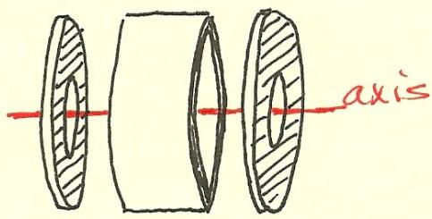
We can use the same formula for both types of segments, based on their width (thickness) & inner & outer radii.
