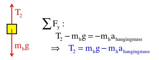
For reasons of clarity, I'm going to redefine this acceleration as the acceleration of the string  $a_{string}$ and rewrite this N.S.L. equation as:  $T_2 = m_h g - m_h a_{string}$   $m_{b}, m_{h}, m_{p}, R, g, \theta, I_{pulley} = \frac{1}{2}m_{p}R^{2}, \text{ and } I_{cm of ball} = \frac{2}{3}m_{b}R^{2}$
