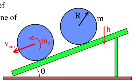
*b.)* What is the velocity of the center of mass after the ball drops a distance *h*.
