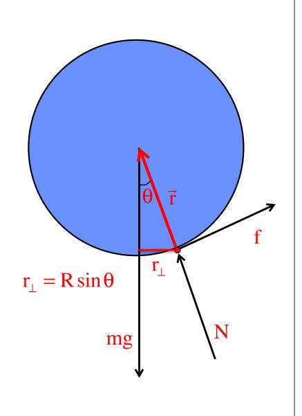
The torque is about the axis at P, so the *moment of inertia* must be about P. Enter (again) the *parallel axis theorem*.
