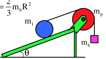
traction, it would spin clockwise), we can take each type of motion, translational and rotational, as a separate entity.
