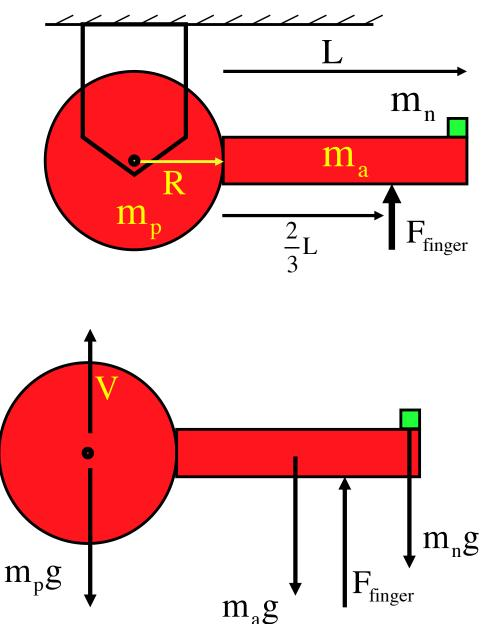
a.) Draw a f.b.d. for the forcesacting on the pulley/arm system.(Hint: Note that as there is only avertical force initially acting at thepin, and there are 5 of these forces).
