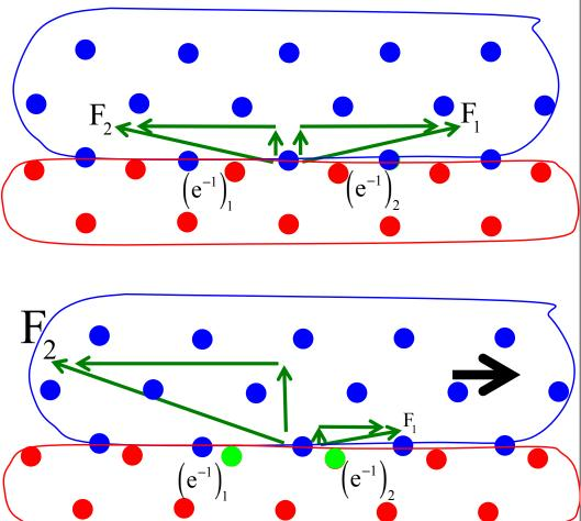
*This net horizontal force* is known as the *static frictional force* between the two bodies. It is the force that has to be overcome before the upper body can actually accelerate to the right. Put a little differently, for the top body to accelerate, an external force to the right that is large enough to effectively shearing the repulsive bonds that exist between electrons has to be applied.
