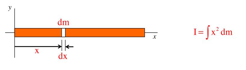
As we did with center of mass problems, we need to relate the position x of the bit of mass to the amount of mass *dm* that is there. To do that, we need to invoke a *density function*.
