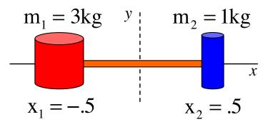
Notice the moment of inertia about the center of mass is smaller than about the other axes denoted. This is always true.  $I_{cm}$  is always a minimum.
