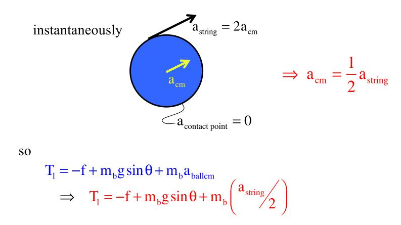
$m_b, m_h, m_p, R, g, \theta, I_{pulley} = \frac{1}{2}m_pR^2$ , and  $I_{cm of ball} = \frac{2}{3}m_bR^2$  *a.*) con't *For ball's rotation* (assuming angular acceleration *clockwise* and summing torques about the center of mass):
