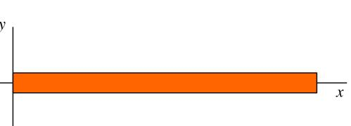
Although this is a continuous mass, the principle is the same. Move out along the x-axis until you find some mass, multiply by the distance-squared, then sum that quantity for all the masses found.
