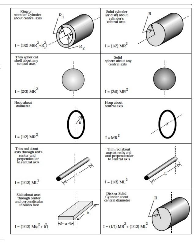
**Example 4:** Remembering what the approach is asking you to do, derive an expression for the moment of inertia of a homogeneous rod of length L about one end.
