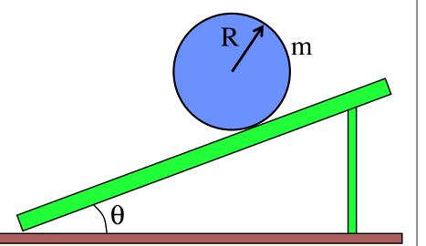
*Before we can do* this problem, there is something that needs to be noted about objects rolling up or down an incline. We need to talk about rolling friction and, more specifically, the direction of rolling friction.
