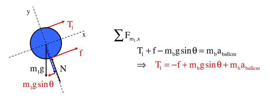
$m_b, m_h, m_p, R, g, \theta, I_{pulley} = \frac{1}{2}m_pR^2$ , and  $I_{cm of ball} = \frac{2}{3}m_bR^2$ The problem with this expression is that we have the hanging mass's *acceleration* in terms of what the string is doing, and the ball's acceleration in terms of what its center of mass is doing. To relate the two, notice that if the
