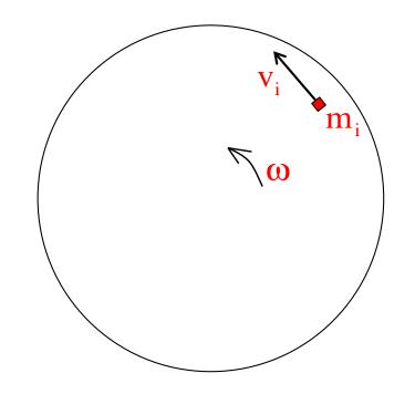
Noting that  $v_i = r_i \omega$ , we can rewrite that summation yielding:  $\mathbf{KE} = \sum_i \mathbf{KE}_i$  $= \sum_i \frac{1}{2} \mathbf{m}_i (v_i)^2$  $= \sum_i \frac{1}{2} \mathbf{m}_i (r_i \omega)^2$  $= \frac{1}{2} \left( \sum_i \mathbf{m}_i r_i^2 \right) \omega^2$
