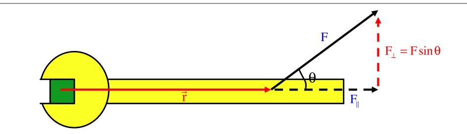
So formally defined, the MAGNITUDE of the torque  $|\vec{\tau}|$  generated by the force on the wrench is mathematically equal to:  $|\vec{\tau}| = |\vec{r}| F_1$
