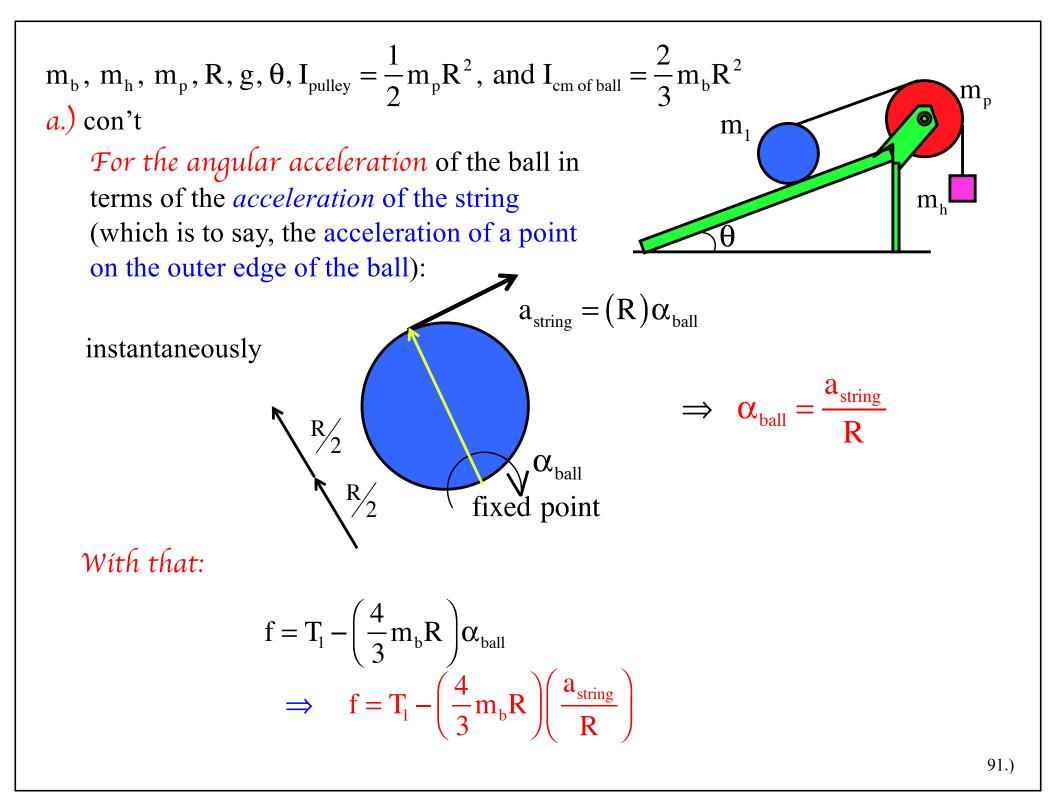
$$m_{b}, m_{h}, m_{p}, R, g, \theta, I_{pulley} = \frac{1}{2}m_{p}R^{2}, \text{ and } I_{cm of ball} = \frac{2}{3}m_{b}R^{2}$$
