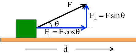
*Clearly,* the perpendicular component of the force  $F_{\perp}$  will do nothing to change the body's velocity (assuming it doesn't yank the block off the tabletop), whereas the parallel component  $F_{\parallel}$  WILL effect a velocity change.
