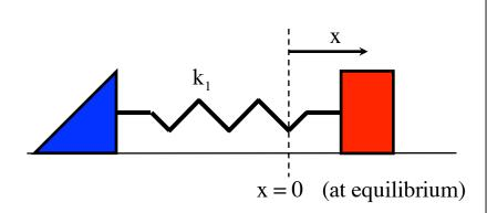
required to elongate or compress the spring  $\ldots$  a big spring constant means a stiff spring—and x is the displacement of the spring from its equilibrium position. In the case of a spring, equilibrium is where the spring force is ZERO.
