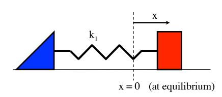
required to elongate or compress the spring  $\ldots$  a big spring constant means a stiff spring—and x is the displacement of the spring from its equilibrium position. In the case of a spring, equilibrium is where the spring force is ZERO.
