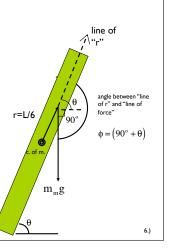
c.) Next is the torque generated by the normal force "V" at the floor, relative to the center of mass. Using the "r-perpendicular" approach (i.e., the product of the magnitude of the "F" vector and the component of "r" that is perpendicular to "F"--this is called "the moment arm," by the way), we get:
