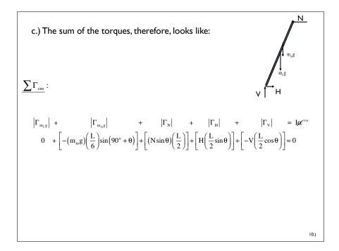
Ν There is an easier way to do all of this. We still have to sum the forces, but if we sum the torques about the floor instead of the center of mass the torques due to m\_g "H" and "V" will be zero and we can ignore them. That leaves torques for only two weights and "N." Using m<sub>L</sub>g the "moment arm" approach (i.e., the rperpendicular approach), each calculations will be н presented below, then the whole things summarized as you would present the material on a test. 12.)
