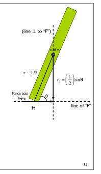
$$\begin{split} \left| \Gamma_{m_{L}g} \right| &+ \left| \Gamma_{m_{m}g} \right| &+ \left| \Gamma_{N} \right| &+ \left| \Gamma_{H} \right| &+ \left| \Gamma_{V} \right| &= Ige^{\pi o} \\ 0 &+ \left[ -(m_{m}g) \left( \frac{L}{6} \right) \sin(90^{\circ} + \theta) \right] + \left[ (N\sin\theta) \left( \frac{L}{2} \right) \right] + \left[ H \left( \frac{L}{2}\sin\theta \right) \right] + \left[ -V \left( \frac{L}{2}\cos\theta \right) \right] = 0 \end{split}$$
