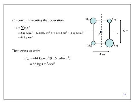
What torque will produce an angular acceleration of 1.5 rad/sec/sec about:
