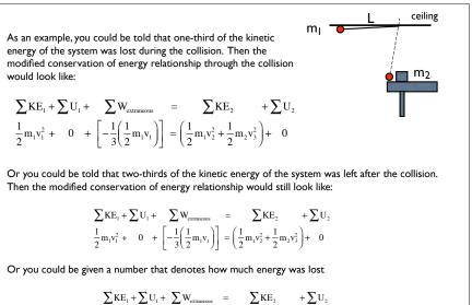
$$\frac{1}{2}m_1v_1^2 + 0 + [-12 \text{ joules}] = \left(\frac{1}{2}m_1v_2^2 + \frac{1}{2}m_2v_3^2\right) + 0$$
