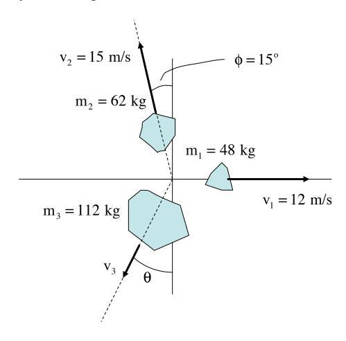
The initial momentum in the system is zero, so the "final" momentum in both the x-direction and y-direction must add to zero. With that in mind, we can write:
