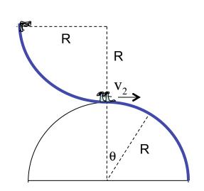
Knowing the velocity after the collision, we can use conservation of energy to determine the velocity just as the two leave the dome. With the mass of the two-body system now "3m," and noting that the distance above the ground at that second point is  $R \cos \theta$ , we can write:
