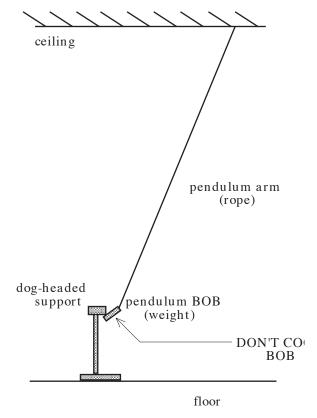
When in position, release the BOB and allow it to swing out into the room, then back to the support. At least five people should eyeball the returning BOB, using the meter stick to visually approximate the final height of the BOB'S *center of mass* at the end of its back swing (due to parallax, everyone should be level with the BOB'S final height). Average the values for all the observers and record that average.
