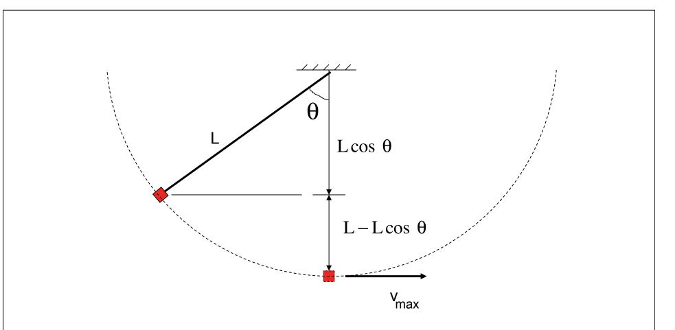
The information provided above will be useful assuming the gravitational potential energy is defined as zero (i.e., y=0) at the bottom of the arc.
