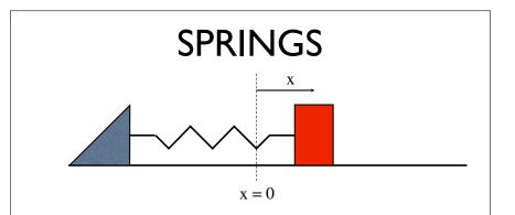
Attach a mass to a spring and push or pull it. If the spring is displaced a distance "x" from its equilibrium position, the spring will exert a force on the mass. The magnitude of that force will be:
