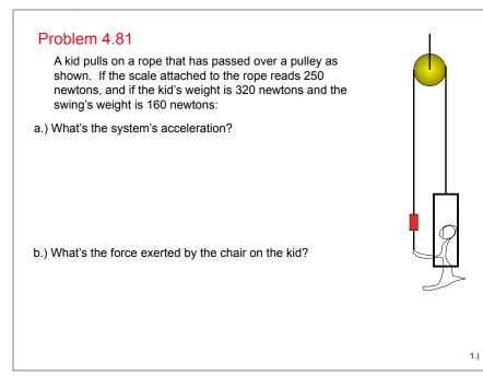
A kid pulls on a rope that has passed over a pulley as shown. If the scale attached to the rope reads 250 newtons, and if the kid's weight is 320 newtons and the swing's weight is 160 newtons:
