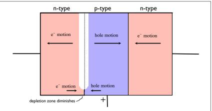
Electrons at the bottom of the left n-type semiconductor will be attracted rightward toward the positive central lead, and similar holes in the p-type semiconductor will be repulsed leftward away from the positive central lead, and the depletion zone at the bottom of the p-n junction will diminish effectively allowing "current" to flow through the circuit and, as a consequence, the load resistor.
