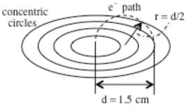
hole and into the upper part of the tube. Once in this region, the electrons collide with an inert gas producing a stream of ionizations and, hence, a blue beam of light. This beam is what will allow you to track the electrons as they pass through the tube.
