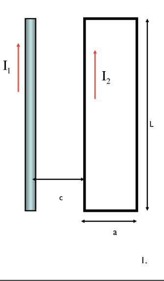
If the left wire current is 5 amps and the loop current is 10 amps, what is the magnitude and direction of the force exerted on the loop by the wire, assuming that a=.15 meters, c = .1 meters and L=.45 meters?
