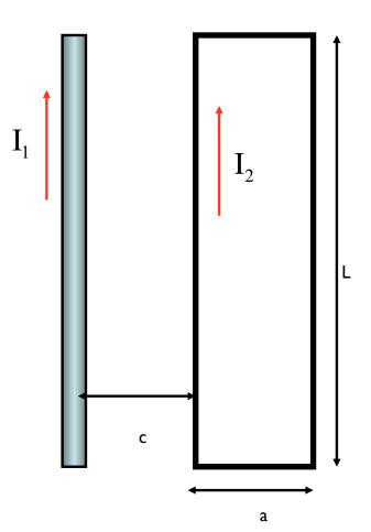
The long wire's magnetic field, using the right thumb rule, is into the page on the right side of that wire. Using the right-hand rule (iLxB), the force directions are shown in the sketch.
