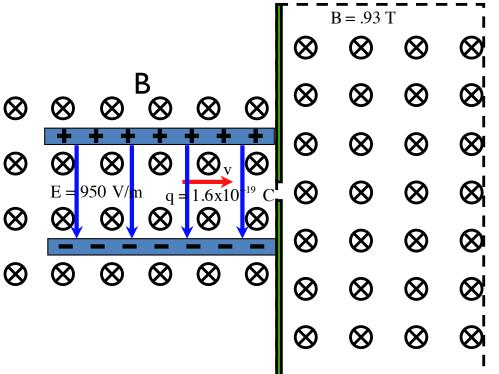
$m = 2.18 \times 10^{-28} \text{ kg}$  E = 950 V/m  $q = 1.6 \times 10^{-19} \text{ C}$ B = .93 T
