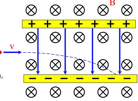
According to the right-hand-rule, a positive charge would feel a force *upward*, so a negative charge will feel a force *downward*.
