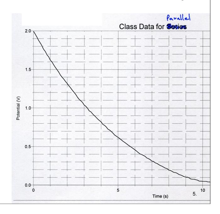
These are discharge graphs for three different capacitances (same resistor in each case). Which cap must have been largest?
