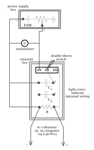
**d.)** After having your circuit checked, turn on the POWER SUPPLY and set the voltage across the capacitor at exactly 2.0 volts as measured using the MULTIMETER.
