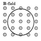
$$\begin{split} \epsilon &= -N \frac{\Delta \varphi_m}{\Delta t} \\ & \Rightarrow \quad \epsilon = -N \frac{\Delta (BA \cos 0^\circ)}{\Delta t} \\ & \Rightarrow \quad \epsilon = -NA \frac{\Delta B}{\Delta t} \\ & \Rightarrow \quad \epsilon = -(50)(.5 \text{ m}^2)(-.4 \text{ teslas/second}) \\ & \Rightarrow \quad \epsilon = 10 \text{volts.} \end{split}$$
