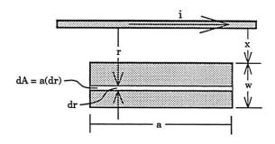
The sketch defines the variables needed. Noting that as the magnetic field vector and area vector are in the same direction, the cosine term in the dot product becomes 1 and the magnetic flux calculation looks like:
