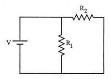
determines how the power function will act. Why? The current is squared in the power relationship. If you halve the resistance of a resistor and its current doubles,  $i^2R$  suggests that the power dissipated by the resistor will double (try the math if you don't believe me). In this case, doubling  $R_1$  will do nothing to  $R_2$  ( $R_2$ 's voltage hasn't changed so its current remains the same, and the power dissipated by  $R_2$  will not change. This response is false.]
