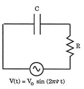
$$\sqrt{{R_{net}}^2 + \left(\!\!\left(\frac{1}{2\pi vC}\right)\!\!\right)^2} = \sqrt{(100\ \Omega)^2 + \left(\!\!\left(\frac{1}{2\pi (80\ hz)(10x10^{-6}\ henrys)}\right)\!\!\right)} = 223\ \Omega. \quad \text{Response is false.}]$$
