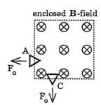
decreasing, so the induced magnetic field will move to fight that decrease by orienting itself in the same direction as the external field. The induced coil current that will effect a magnetic field through the coil in that direction will be clockwise. This response is false.]
