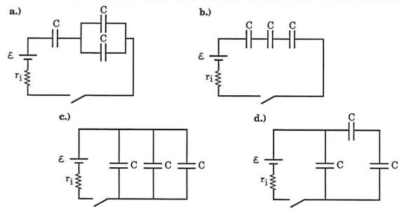
a.) Circuit a. [This is a bit tricky. The uncharged capacitors act like shorts when the switch is thrown. That is, current effectively passes through them without any resistance to charge flow whatsoever. As such, we could as well remove all of the capacitors from the circuit and replace them with simple wires. As wires are theoretically assumed to have no effective
