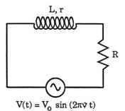
impedance at the frequency of operation. We have already established that the inductive reactance doubles with a doubling of the frequency, but how does the circuit's net resistive nature--its impedance--change? The impedance expression for an RL circuit is
