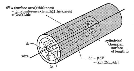
NOTE: The hollow's radius should be "a" while the outside radius is "2a". The sketch is NOT to scale to afford you a better look at the Gaussian cylinder, etc.
