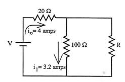
Kirchoff's Laws. Starting with the voltage, all you need to notice is that the voltage drops across the  $20~\Omega$  and  $100~\Omega$  resistors have to add to the voltage across the battery. Using that information, we can write  $V = (20~\Omega)(4~amps) + (100~\Omega)(3.2~amps) = 400~volts$ . From that information alone, this response is false.]
