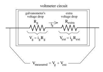
deflection, the voltage drop across the galvanometer will be its maximum deflection current times its known resistance, or  $(5x10^{-4} \text{ amps})(R_g)$ . Let's say the galvanometer's resistance is 20 ohms. The voltage across the galvanometer at full deflection will, therefore, be  $10^{-2}$  volts. Unfortunately, we want the galvanometer's needle to move full deflection when 5 volts is placed across the meter. So how do we insure that this
