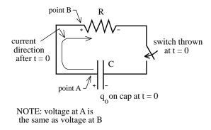
around the closed loop have to add to zero (i.e., she knows Kirchoff's Laws), so she starts on the right side of the capacitor and traversing clockwise. She observes a voltage increase across the capacitor of q/C and a voltage drop across the resistor of iR (see circuit). With that, she writes:
