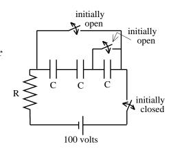
circuit and a third capacitor is plated in series with the other two caps. Because the capacitors are all the same size, you would expect the charge to distribute itself evenly between the three. That means the charge on one cap will be  $(1/3)(CV_o/2) = CV_o/6$ .
