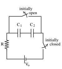
difference between the caps. Current will flow until that voltage difference disappears.
