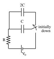
a.) What is the voltage across the second capacitor? <u>Solution</u>: Charge will flow until there are no more voltage differences in the circuit. That is, half the voltage will be across the first cap and the other half across the second cap.
