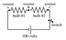
a.) *Bulb* #1 is taken out of the circuit by putting a wire across terminals A and B.
